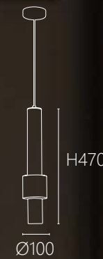
OK 21491 36000 Ø100 H470mm 線長1500mm LED 5W x 1 / MR16 x 1 3000K 鋁材
